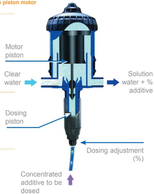
Therefore, the operating principle ensures constant dosing, independently of the variations in flow rate and pressure of the water.
